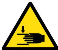
**Crushing hazard.** Keep hands away from moving machine parts or wait until all moving parts have stopped.
